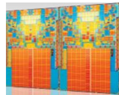
Intel Itanium 9150 (x64) Multi Processors (2) 1.7 Billion Transistors
